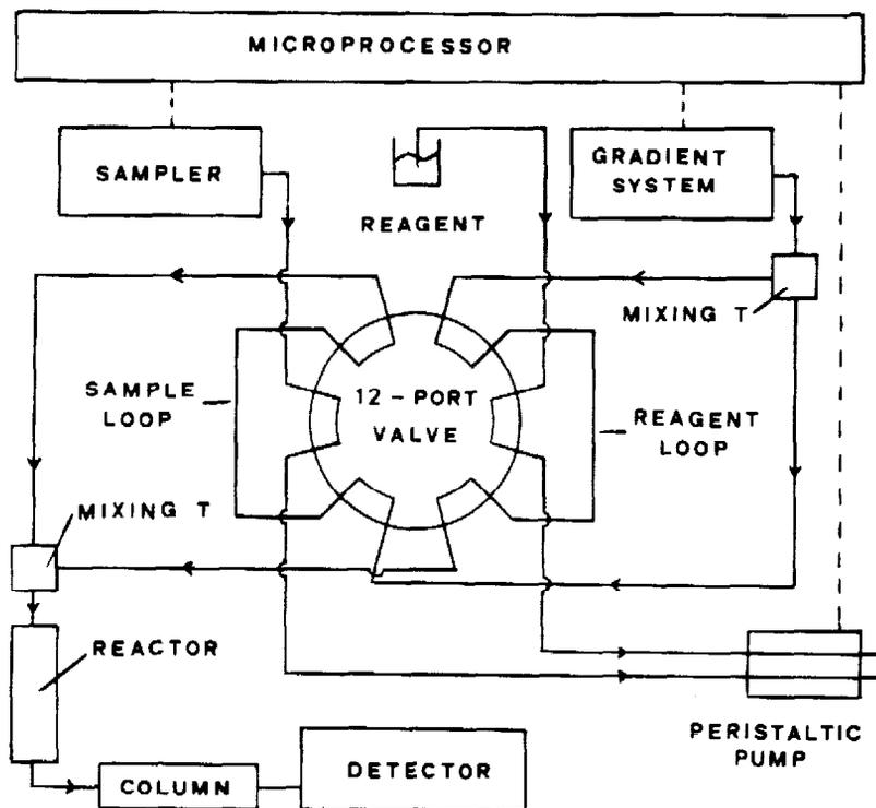
Fig. 1. Automated pre-column derivatisation device; twelve-port valve shown in "inject" position.
